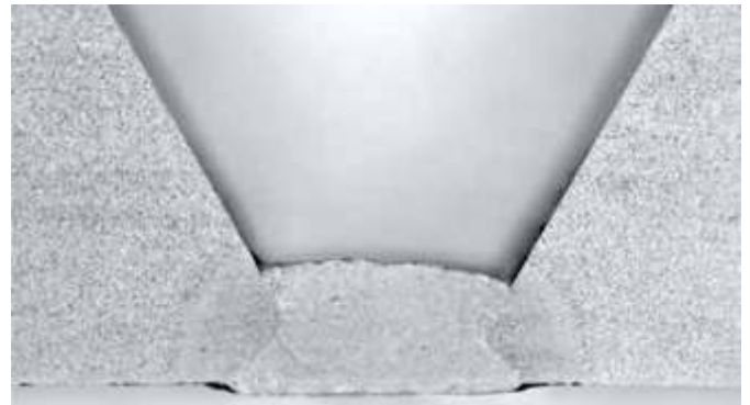
PG - Butt Weld S355 - THK 3mm - GAP 1.5 mm
